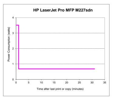
The device is so designed as to ensure that it can be switched to the Plug-in Off mode by pressing the on/off switch up to twice a day without suffering damage. This device does not have a switch by which it can be completely disconnected from the mains. When after having switched off the device you pull out the power plug, electric power consumption is completely stopped.
